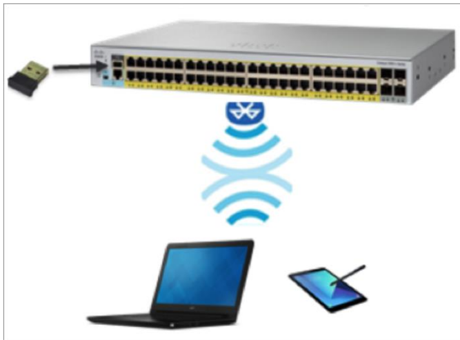
Figure 2. Over-the-air switch access using Bluetooth
